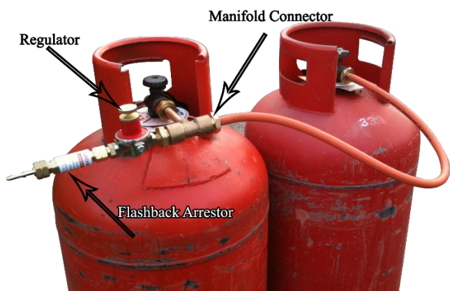
Propane Bottles Correctly Coupled together
