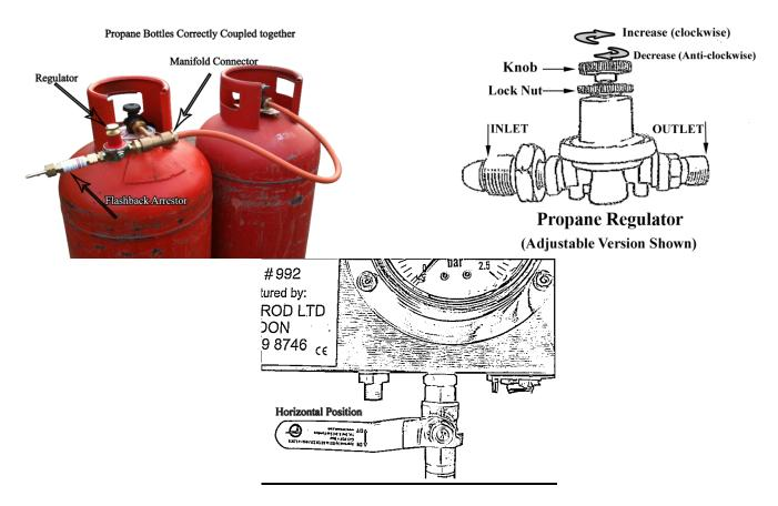
Ensure that main burner tap is in the off position i.e., horizontally across the tap is off - in line with the tap vertically is on.
